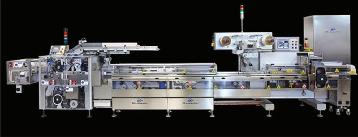
PFM provides an automatic high-speed line equipped with feeding system, product counting device<sup>1</sup>, shingling unit<sup>2</sup> and transfer system<sup>3</sup> to convey the product onto the wrapper's infeed conveyor.
