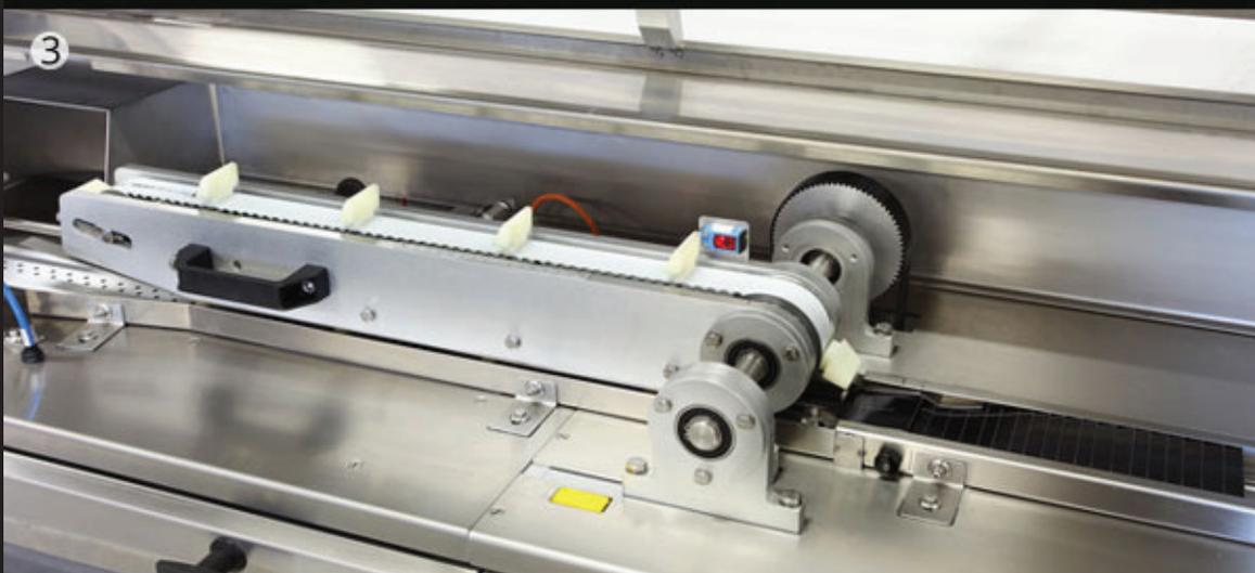
The cartoning machine accepts perfume vials from the filling line and inserts them into the U Fold cards. By means of the automatic system supplied by PFM the single cards are subsequently inserted one inside the other produce the various formats comprising of 5 to 20 pieces which are then collated and transferred to the [PFM FALCON HS](#) wrapper, a completely servo controlled machine. A set of sensors specifically dedicated to the product formats allows reject packs to be discarded.
