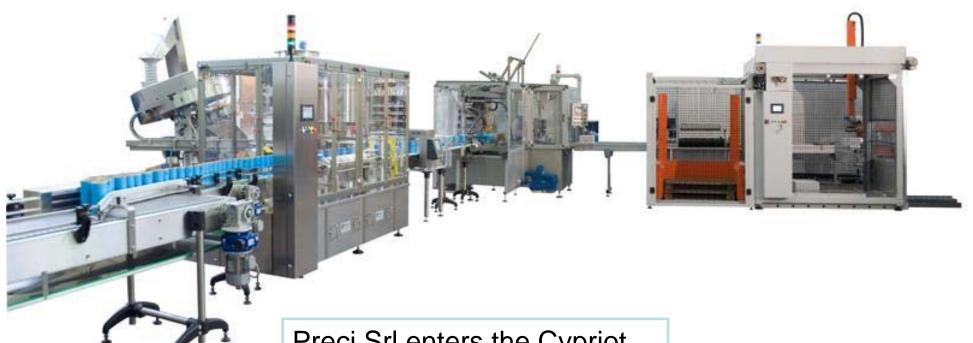
Preci Srl enters the Cypriot market with a state-of-the-art salt packaging line, to pack dry, free flowing fine and coarse table salt into rigid containers.
