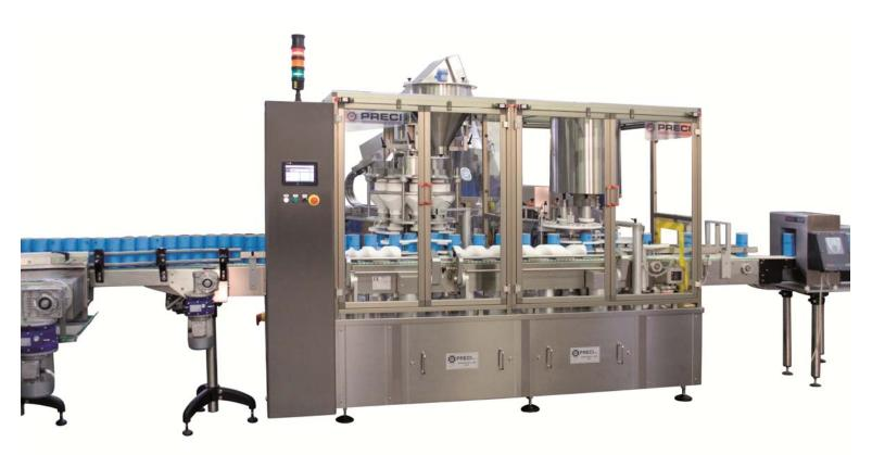
Simple and quick size changeover facilities and easy parts removal for cleaning.
